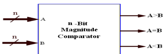
Figure 1. Block Diagram of n-Bit Magnitude Comparator
