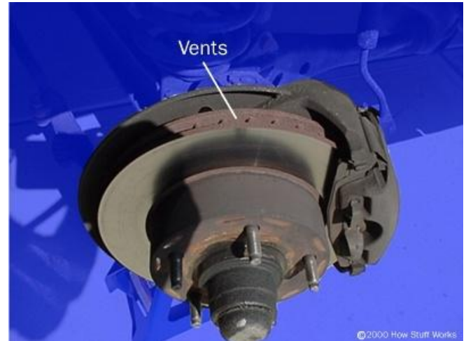
Fig -2: Vents provided on Disc Brakes
