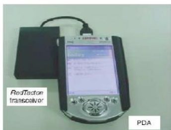
Fig.3. shows a photograph of the RedTacton transceiver connected to a PDA.
