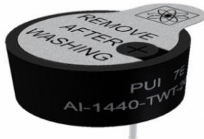
Fig.3.7 Replicate of Buzzer Image Used In PCB
