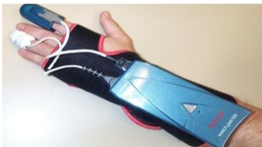
Fig 2.6 shows ambulatory recording system consisting of two finger sensors for the peripheral arterial tonometry and for the pulse oximetry
