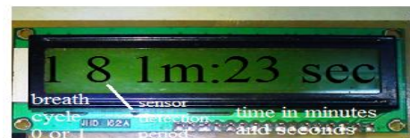
Fig 3.4 LCD display Showing breath cycles per minute
